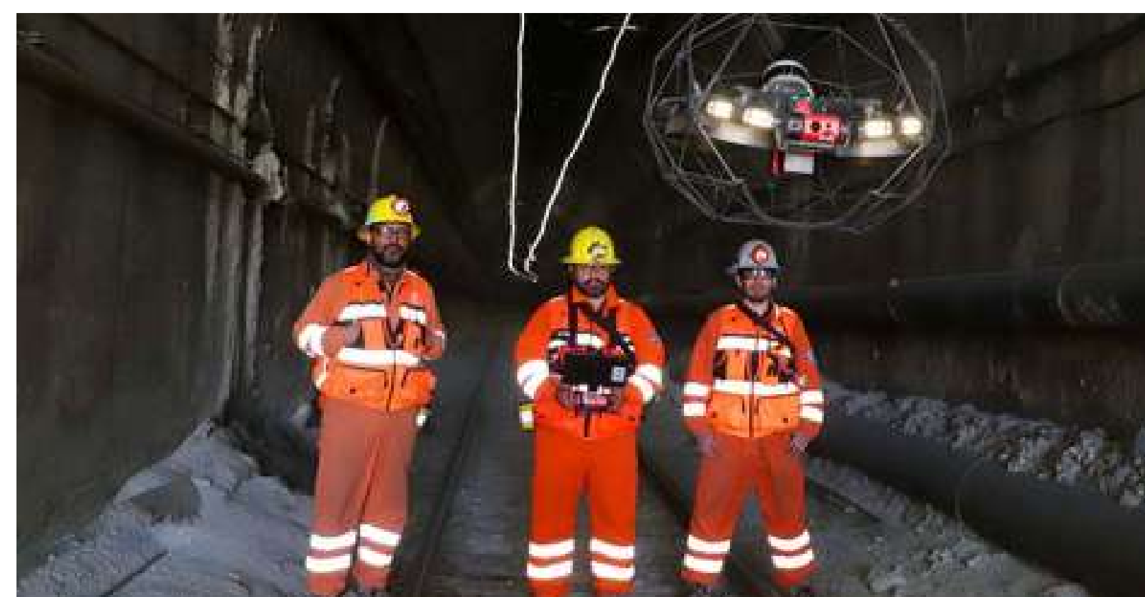
Flyability – 3D tunnel mapping using drones at El Teniente, Chile
