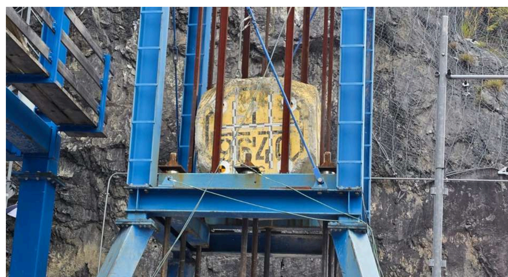
Geobrugg – Dynamic testing of tunnel support systems at the Walenstadt test facility
